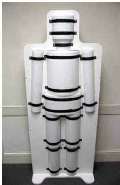
Figura 2. 8 Fantoma BOTTle Manikin Absorber (BOMAB). (ICRP 23).
